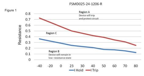
IH (I Hold) defined as the maximum current the device will hold at rated temperature (23°C) without tripping. The probability that the PPTC will trip increases as the current approaches IT (I Trip), defined as the minimum current required to cause the PPTC device to trip at rated temperature.
