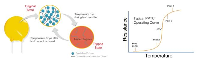
If the device is operated above IH, but under IT at rated temperature, depends on the initial resistance, the heat could still accumulated inside PPTC and reach trip temperature after a longer period of time.
